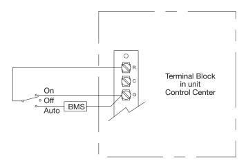
Hand/Off/Auto Switch allows the unit to
